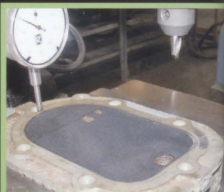
Mr. Sands milling the head on his garden tractor pull motor to try on get more compression out of it.
